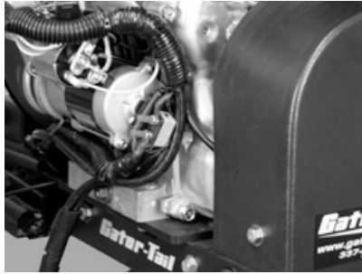
Breaker located near rear of starter
